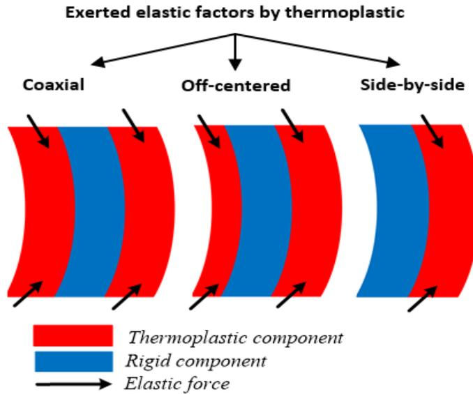
Figure 7. Schematic diagrams of elastic forces of thermoplastic component exerted on the helical nanofibers. After from, after from. <sup>57</sup>
