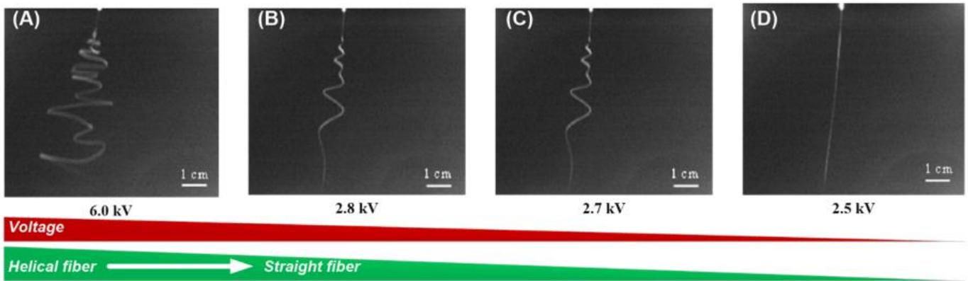
Figure 5. The effect of applied operating voltage on the helical structures formation. (A) 6.0 V, (B) 2.8 V, (C) 2.7 V, (D) 2.5. Reproduced from
