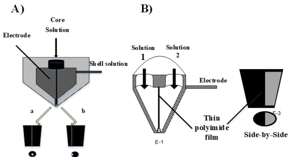
**Figure 6.** Shows a schematic diagram of electrospinning spinnerets with a bicomponent feed (A) coaxial (a), off-centered (b) and (B) side-by-side electrospinning spinnerets, after from
