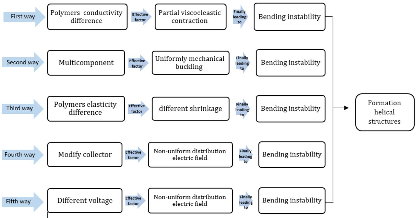
Figure 9. Different ways of affecting the mechanical parameters on the formation of the helical structures
