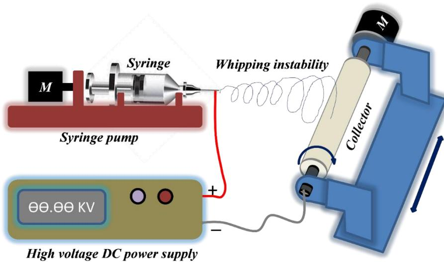
Figure 4. Schematic setup of an electrospinning process
