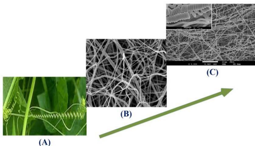
Figure 2. Comparison of the plant tendrils (A), straight (B) and helical nanofibers (C), reproduced from
