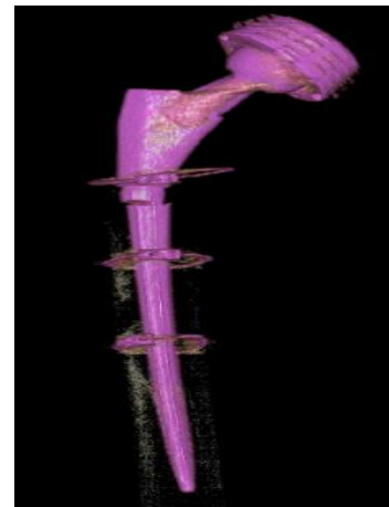
Figure 5. Preliminary CT-scan (3D reconstruction) of the second prosthetic modular stem fracture (2023)
