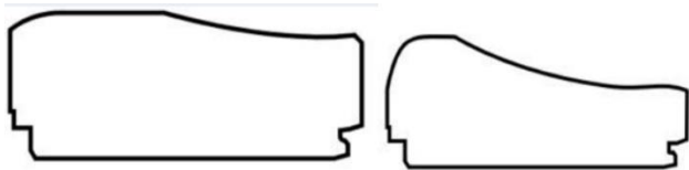
Figure 1. SIGMA Polyethylene designs Curved (CVD) (left) and Curved Plus (CVD+) with increased anterior lip height (right)
