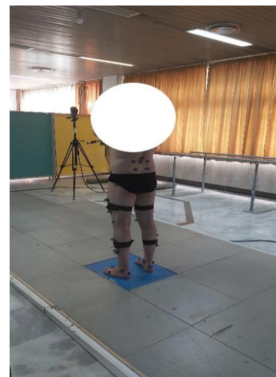
Figure 1. The person's status and marker placement during static "StTS" test recording
