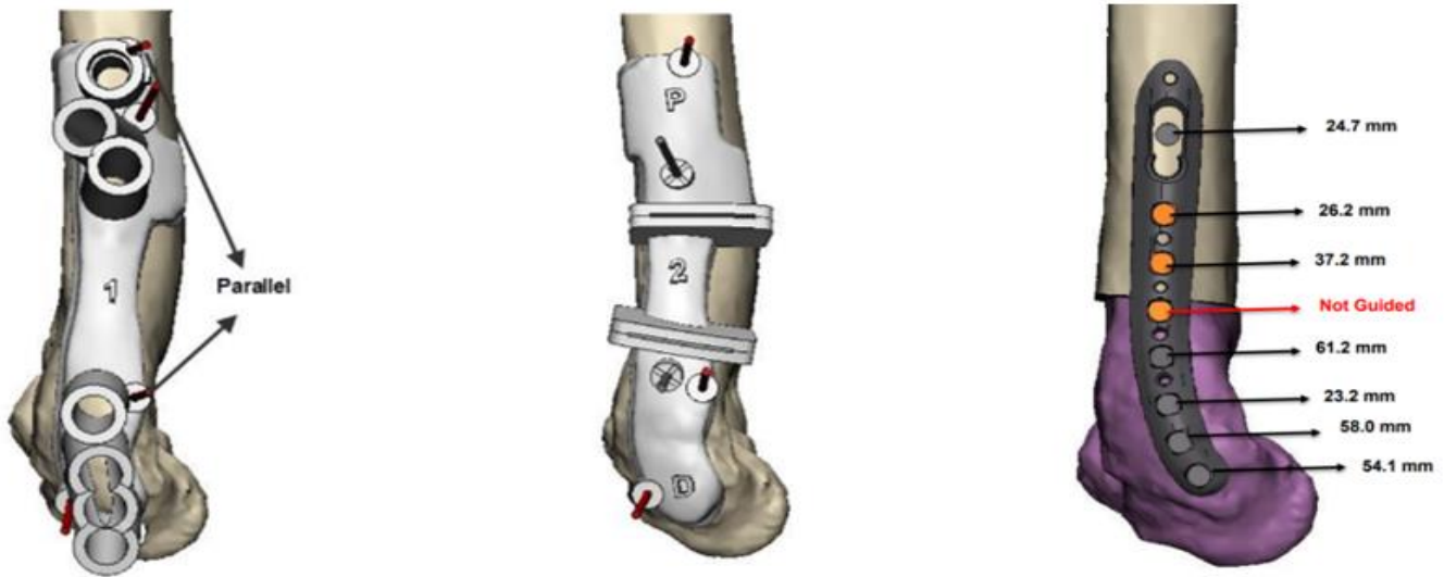
Figure 1. Example of 3D planning of a distal humeral correction osteotomy. From left to right: a screw hole drill guide, a sawblade guide and planned plate and screws
