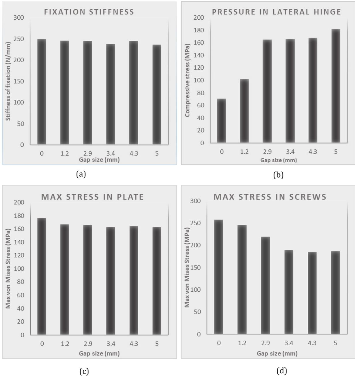
**Figure 4.** Effect of the level of anatomical fit of the TomoFix plate on (a) Stiffness of fixation, (b) Lateral hinge pressure, (c) Maximum equivalent stress in plate, and (d) Maximum equivalent stress in screws.
