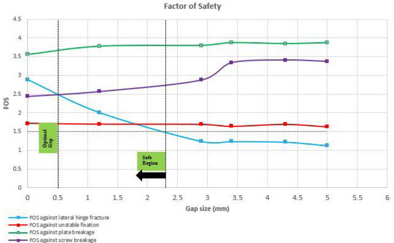
**Figure 5.** Factor of safety-level of anatomical fit diagram of High Tibial Osteotomy fixation using TomoFix plate. The safe region includes the range of the anatomical fit with a factor of safety higher than 1.5 against all four modes of failure. The optimal state (gap=0.5 mm) indicates the anatomical fit with the highest possible factor of safety for all four modes of failure.
