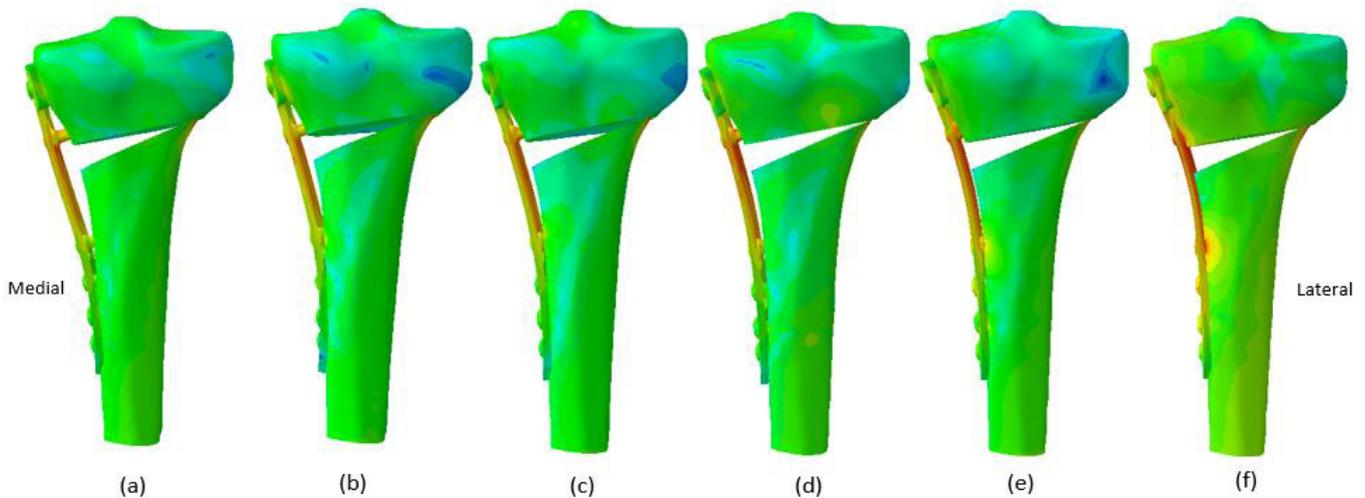
Figure 3. Results of the finite element model for the six states of the anatomical fit: (a) 5 mm gap, (b) 4.3 mm gap, (c) 3.4 mm gap, (d) 2.9 mm gap, (e) 1.2 mm gap, and (f) zero gap.
