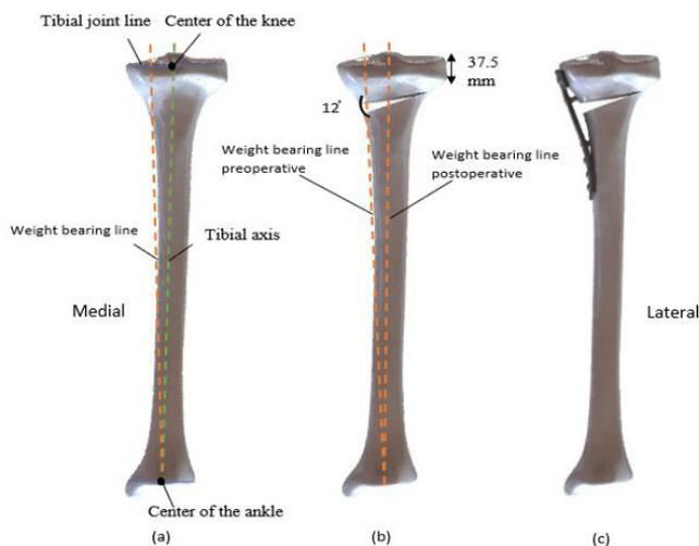
Figure 1. Simulation of open-wedge High Tibial Osteotomy: (a) Original tibia with varus orientation, (b) Simulation of the High Tibial Osteotomy operation, and (c) TomoFix plate fixation of High Tibial Osteotomy.
