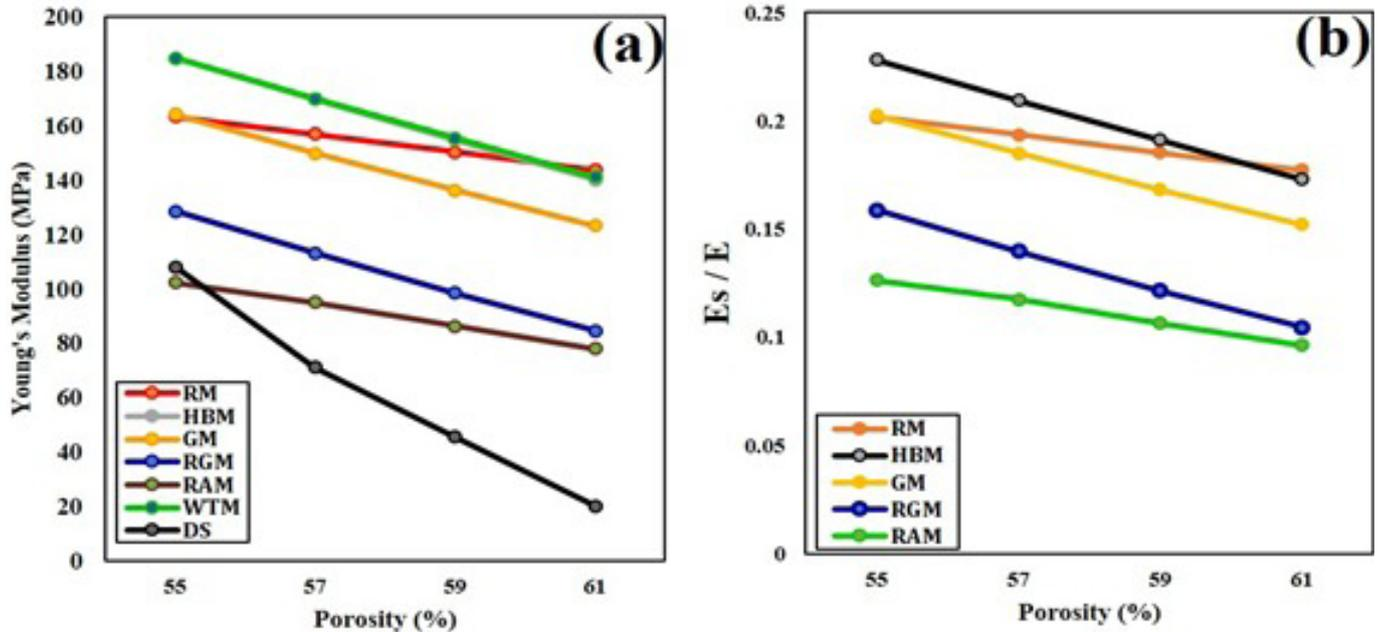
Figure 5a, b. Micromechanical model used to predict the compressive strength of various porous architecture (a) elastic modulus vs. porosity, (b)  $E_s/E_p$  vs. porosity value for bio-nanocomposite with various amount of SWCNT.
