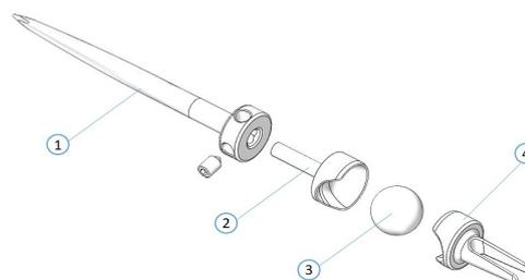
Figure 1. Intraosseous DRUJ prosthesis components: 1- Proximal stem, 2- Locking segment including a proximal concave unit, 3- Globe, and 4- Distal stem including a distal concave unit.
