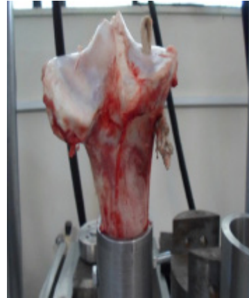
Figure 2. The Achilles grafts are fixed with biodegradable interference screws and bone plug on tibia with both ends (9*30).
