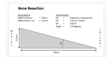
Figure 2. An illustration of the effect of a 1.2mm differential bone cut between medial (more) and lateral (less) compartments of the knee that results in a 1 degree change in alignment (varus)
