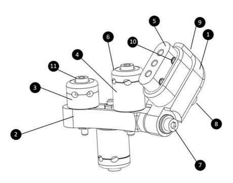
Figure 2. Dynamic External fixator components: 1: Head, 2: Semi-lunar part, 3: Short rod, 4: Long rod, 5: Sliding core, 6: Pulley, 7: Semi-lunar part-head connecting screw, 8: Compression screw, 9: Above the head screw, 10: Nutting screw, and 11: Rod screw
